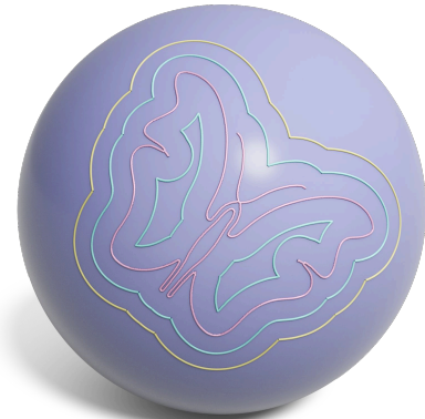
Figure 1: Offset curves on a spherical parametric surface. The source curve (shown in pink) and its offset curves at two different distances (shown in cyan and yellow, respectively) are illustrated on the spherical surface.
